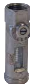
FLOW METER with Mechanical Regulation BSP 1/2" (Female) - BSP 3/4" (Male) Hexagonal: SW19 Full Length: 81mm Flow capacity: 2 - 8 lt/min Temperature Range: +0°C - +100 °C Working Pressure: max 10 Bar Springs: Stainless Steel Indicator Plastic Seals: Buna Article number: FM 1234
