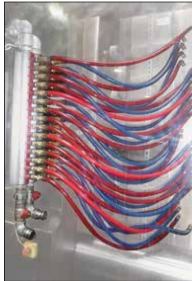
DME cooling manifold
